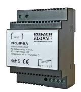
The PSICL Series is a range of inrush current limiters designed to protect against unintended fuse or circuit breaker activation caused by peak currents. The benefits can result in reduced cable cross section and the use of smaller and faster circuit breakers. These are not simple NTC devices and feature current control circuits with integrated bypass relays.
