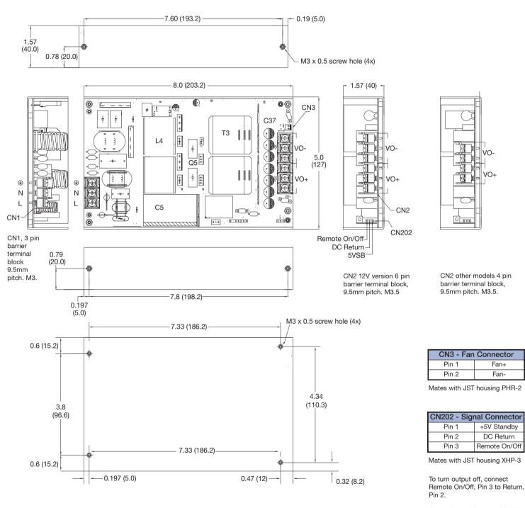
Output is on if Remote On/Off, Pin 3 is floating or connected to 5V standby, Pin 1.
